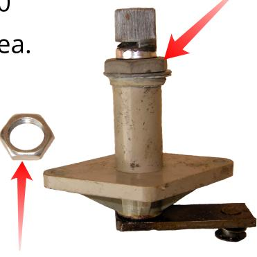
[ New Steel Securing Nut ]
