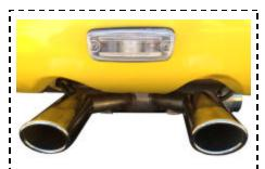
**Rear Resonator** Rounded baffled oval tips, provide a modern design and smooth sound
