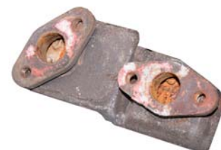
Original Opel GT Heater Core Like the original radiators, the cores get clogged with trapped corrosion and iron sediment
